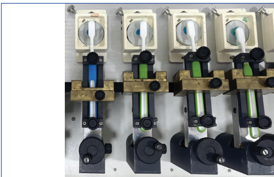
[Table/Fig-1]: Brushing simulator showing 4 samples tested using soft-bristled toothbrush and fluoridated toothpaste under a consistent pressure of 3 N.
